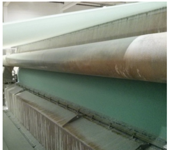
Primoselect high speed gap former cleanliness
