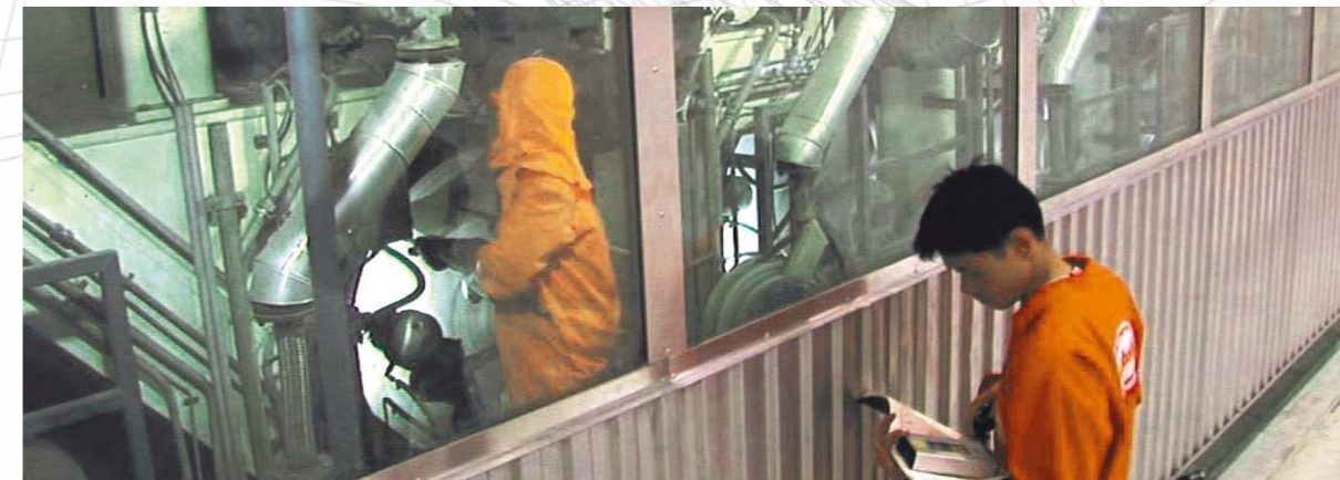
Fig. 5: Temperature measurement in the dryer hood
